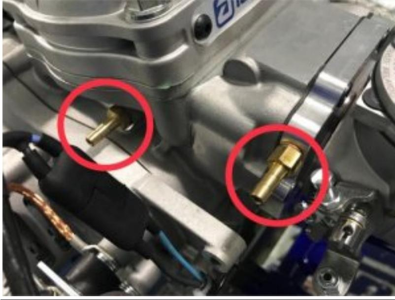
Connect a pulse tube between the two fittings as shown
