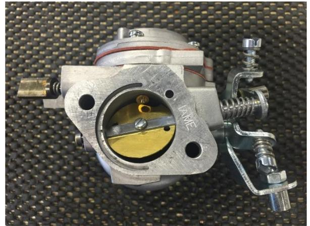
Picture above shows butterfly without “dimples”, and shows butterfly in slightly open position if not tightened properly.
