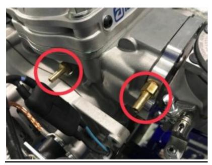
Connect a pulse tube between the two fittings as shown
