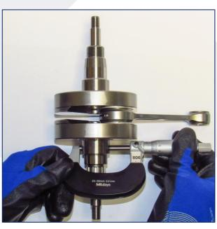
The crankshaft and the micrometer have to be at the same ambient temperature.
