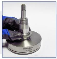
Install the bearing spacer. The side with the marking must <u>face down</u> toward the crankshaft body.
