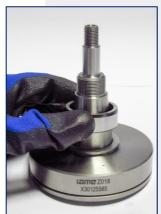
Place the inner ring onto the crankshaft, the marking must <u>face down</u> toward the crankshaft body, while the bigger chamfer must <u>face upwards</u> and remain visible.
